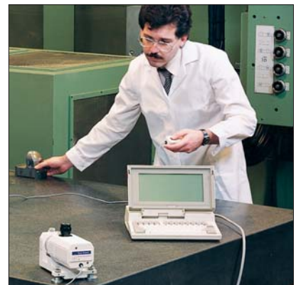
Checking surface table flatness with a DA400 Autocollimator
