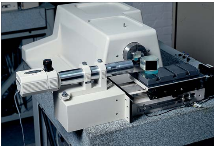
Precision Machine Tool alignment using DA20 Autocollimator
